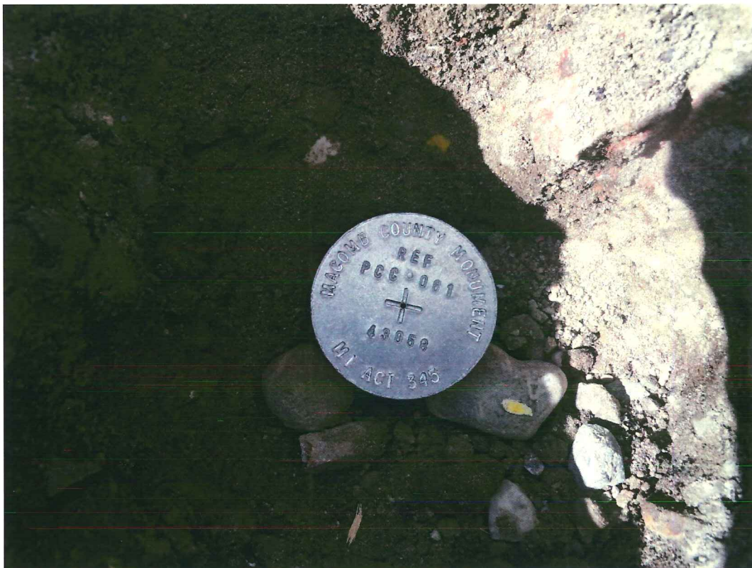
AFTER – Reference to PCC-061. Set 3/4"x24" iron with disk. (05/29/2014)
