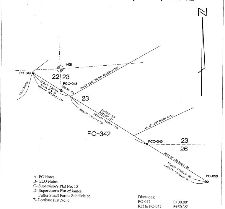
SECTION LINE MEASURED DURING GLO SURVEY AZIMUTH & LENGTH USED FOR INDEXATION
