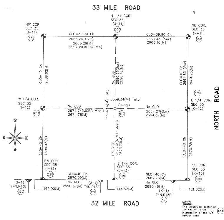
SECTION 35, T5N,R13E ARMADA TOWNSHIP (96-4013) J-12 (as found) to the theoretical center of the section is N32'27'17"E 12.18 REMSED: 5/23/01
