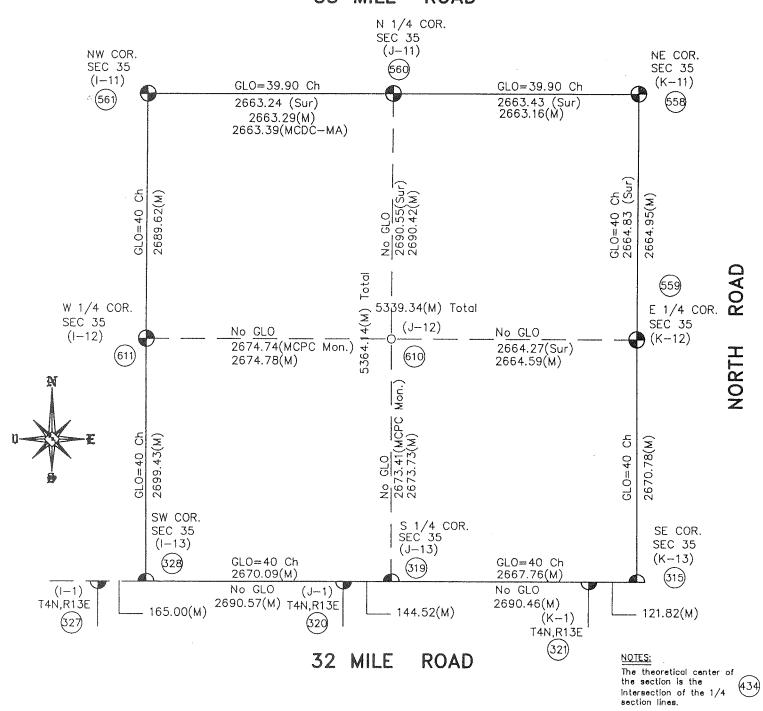
SECTION 35, T5N,R13E ARMADA TOWNSHIP (96-4013) J-12 (as found) to the theoretical center of the section is N32'27'17"E 12.18 REMSED: 5/23/01
