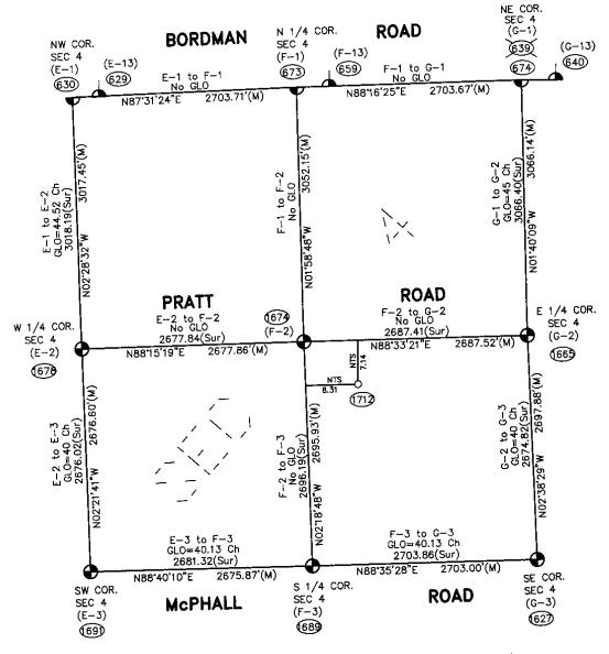
Theoretical Center of Section is at the intersection of the theoretical lines between the 1/4 corners.
