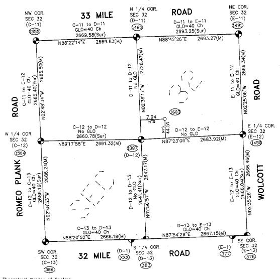
Theoretical Center of Section is at the intersection of the theoretical lines between the 1/4 corners.
