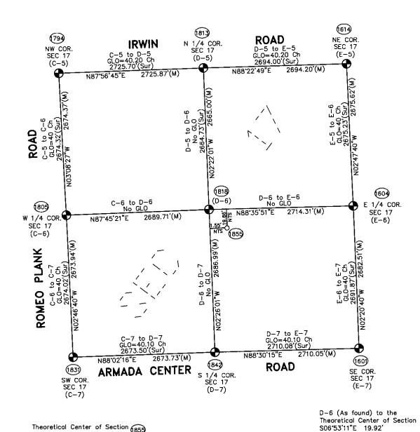
Theoretical Center of Section is at the intersection of the theoretical lines between the 1/4 Section Lines.
