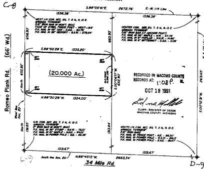
I HEREBY CERTIFY THAT I HAVE SURVEYED THE PARCEL(S) OF LAND DESCRIBED AND DELINEATED HEREON; THAT SAID SURVEY WAS PERFORMED WITH A RELATIVE ERROR OF CLOSURE NO GREATER THAN I' IN 5,000'; AND THAT I HAVE FULLY COMPLIED WITH THE REQUIREMENTS OF SECTION 3, ACT 132, P.A. 19/0, AS AMENDED.
