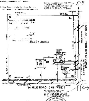
I hereby certify that I have surveyed the parcel(s) of land described and defineded hereon; that said Survey was performed with an error of closure no greater than I in 5,000; and that I have fully complied with the requirements of Section 3, Act 132, P.A. 1970.
