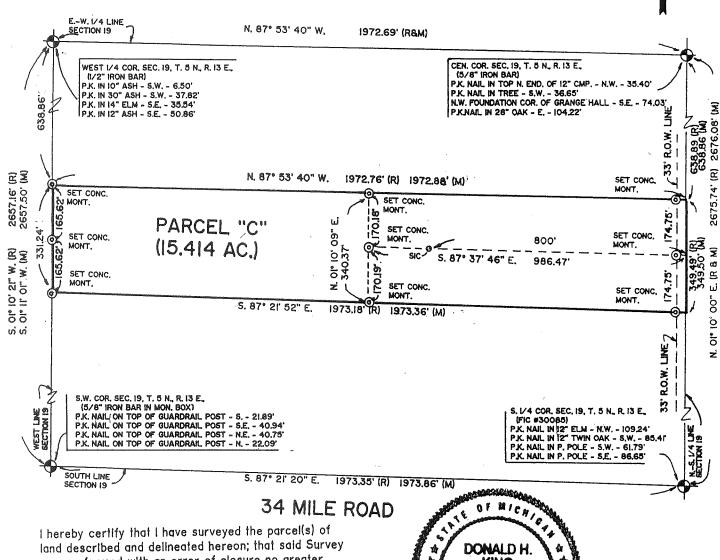
I hereby certify that I have surveyed the parcells, or land described and delineated hereon; that said Survey was performed with an error of closure no greater than I' in 5,000'; and that I have fully compiled with the requirements of Section 3, Act 132, P.A. 1970.
