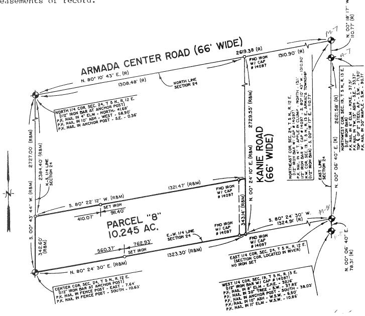
I hereby certify that I have surveyed the parcel(s) of land described and delineated hereon; that said Survey was performed with an error of closure no greater than I' in 5,000'; and that I have fully complied with the requirements of Section 3, Act 132, P.A. 1970.
