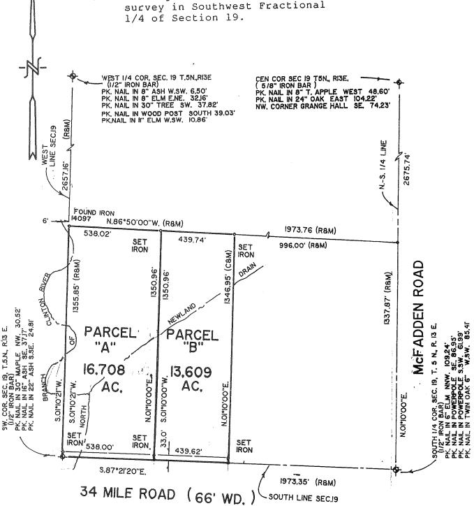
I hereby certify that I have surveyed the parcel(s) of land described and delineated hereon; that said Survey was performed with an error of closure no greater than 1 in 5,000; and that I have fully complied with the requirements of Section 3, Act 132, P.A. 1970.
