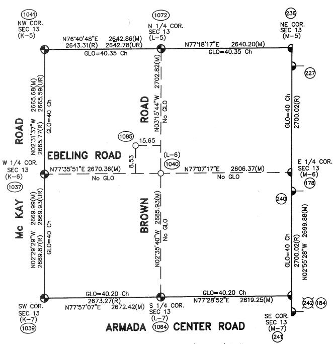
Theoretical Center of Section ( the intersection of the 1/4 Section Lines) L-6 (As Found) to the Theoretical Center of Section N64°40'34"W 17.82'
