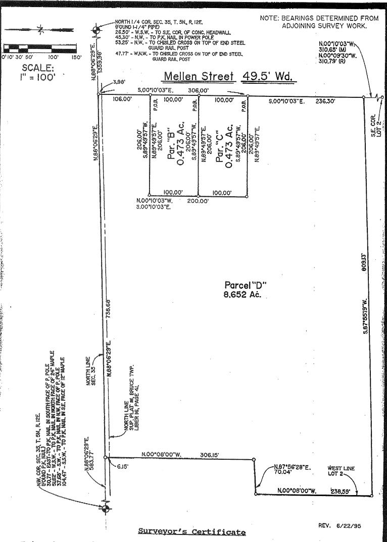
hereby certify that I have surveyed and mapped the land above platted and/or described on June 7, 1993 and that the ratio of closure on the unadjusted field observations of such survey was 1/93,755 and that all of the requirements of P.A. 132 1970 have been complied with.
