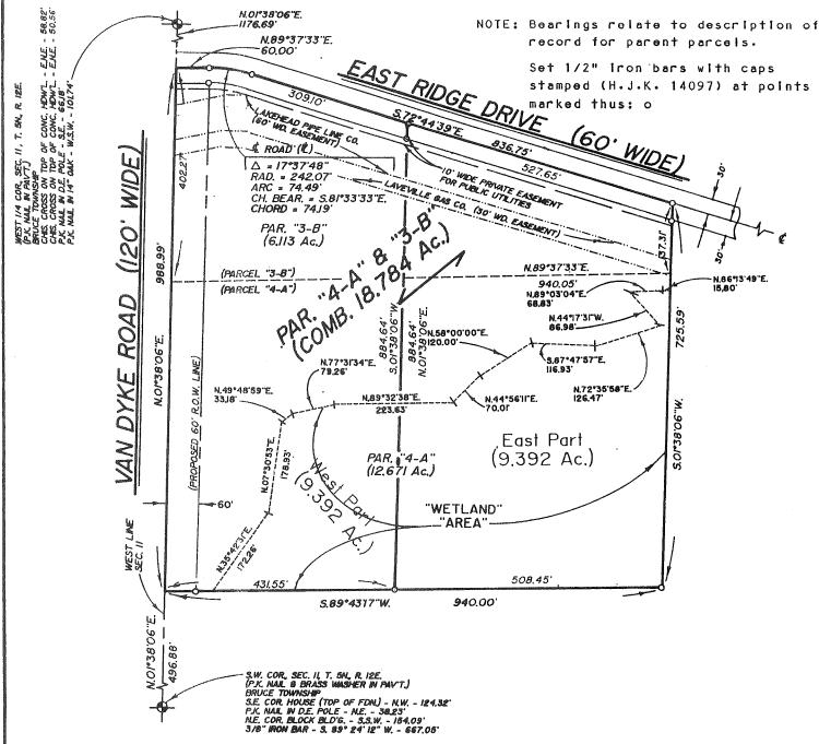
I hereby certify that I have surveyed the parcel(s) of land described and delineated hereon; that said Survey was performed with an error of closure no greater than I in 5,000; and that I have fully complied with the requirements of Section 3, Act 132, P.A. 1970.
