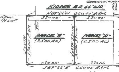
I HEREBY CERTIFY THAT I HAVE SURVEYED THE PARCEL(8) OF LAND DESCRIBED AND DELINEATED HEREON; THAT SAID SURVEY WAS PERFORMED WITH A RELATIVE ERROR OF CLOSURE OF 1 IN 11,1251; AND THAT I HAVE FULLY COMPLIED WITH THE REQUIREMENTS OF SECTION 3, ACT 132, P.A. 1970.
