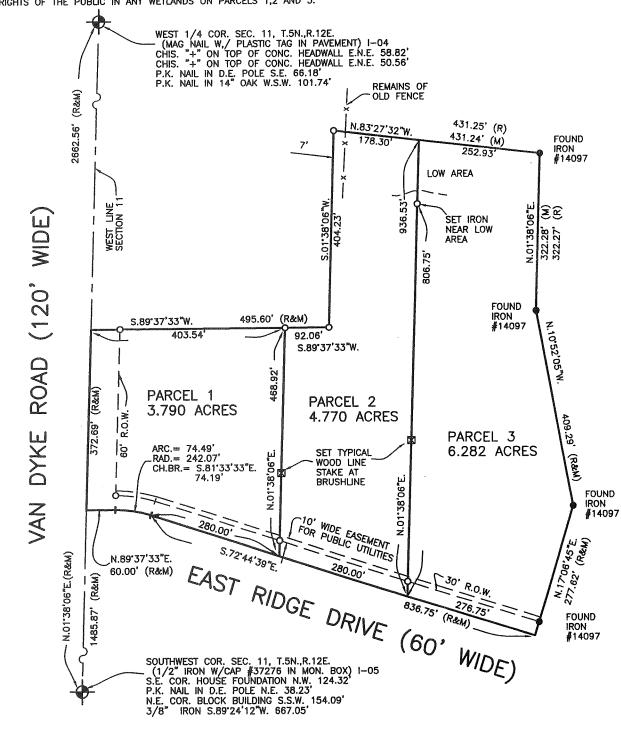
I hereby certify that I have surveyed the parcel(s) of land described and delineated hereon; that said Survey was preformed with an error of closure no greater than 1 in 5000; and that I have complied with the requirements of Section 3, Act 132, P.A. 1970 as ammended.
