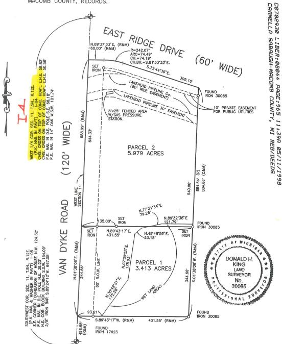
I hereby certify that I have surveyed the parcel(s) of land described and delineated hereon; that said Survey was preformed with an error of closure no greater than 1 in 5000; and that I have complied with the requirements of Section 3, Act 132, P.A. 1970 as ammended.
