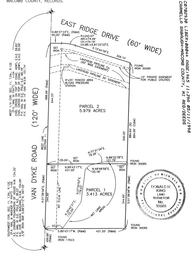
I hereby certify that I have surveyed the parcel(s) of land described and delineated hereon; that said Survey was preformed with an error of closure no greater than 1 in 5000; and that I have complied with the requirements of Section 3, Act 132, P.A. 1970 as ammended.
