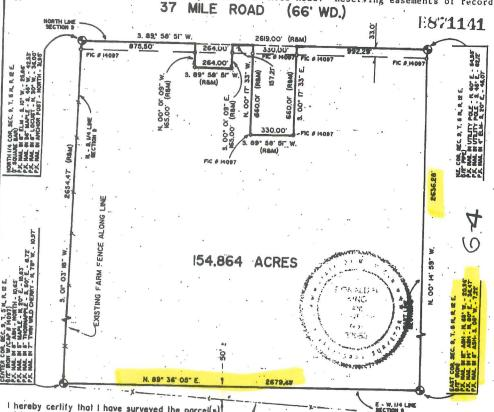
I hereby certify that I have surveyed the parcel(s) of land described and delineated hereon; that said Survey was performed with an error of closure no greater than I' in 5000 and that I have fully complied with the requirements of Section 3, Act 132, P.A. 1970.
