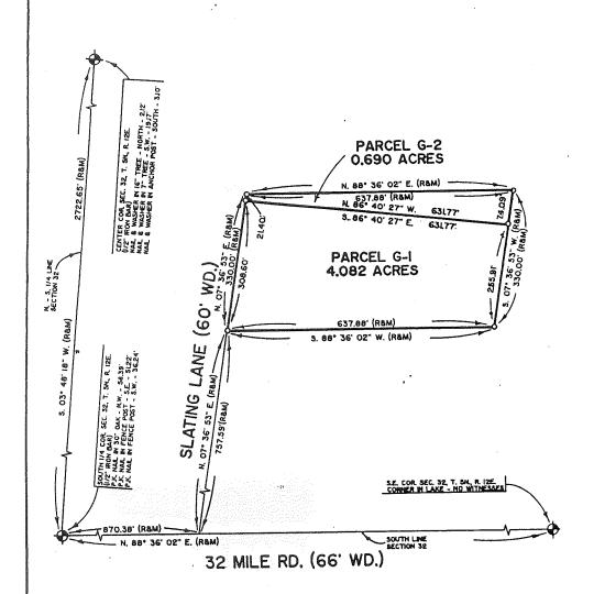
I hereby certify that I have surveyed the parcei(s) of land described and delineated hereon; that said Survey was performed with an error of closure no greater than I in 5,000; and that I have fully compiled with the requirements of Section 3, Act 132, P.A. 1970.
