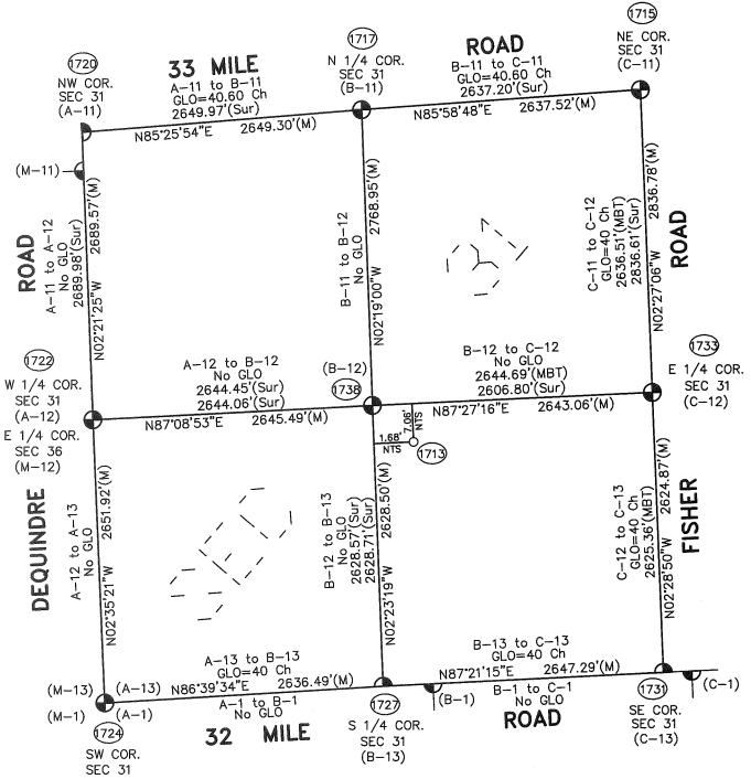
Theoretical Center of Section (713) is at the intersection of the theoretical lines between the 1/4 Section Lines.
