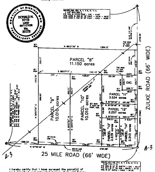
I hereby certify that I have surveyed the parcel(s) of land described and delineated hereon; that said Survey was performed with an error of closure no greater than 1' in 5,000'; and that I have fully complied with the requirements of Section 3, Act 132, P.A. 1970.
